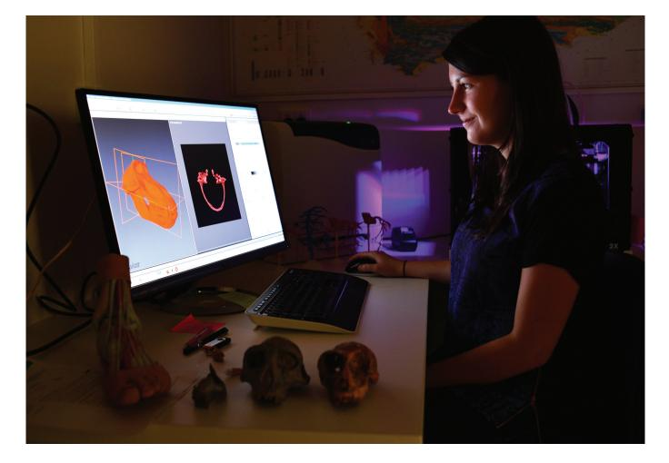
Through MASSIVE research have access to a high-performance desktop environment. Data stored on MASSIVE can be analysed using interactive desktop tools underpinned by a fast parallel file system, high memory and fast GPU rendering.
